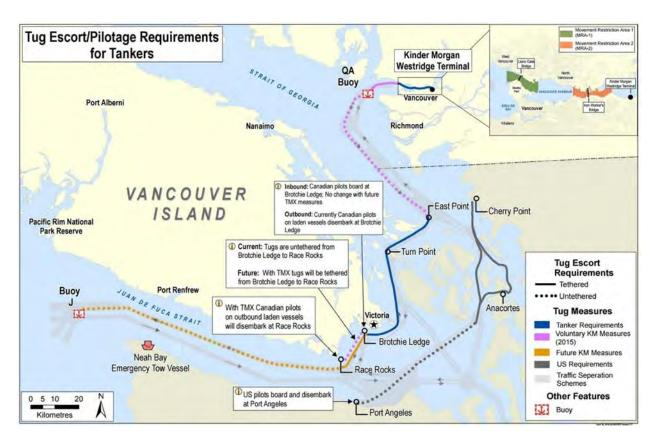
Figure 28 - Tug escort/pilotage requirements for tankers Source: TC
