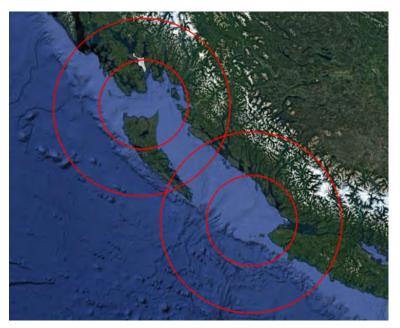
some cases when an EOTV is within 8 hours (128 NM at a speed of 16 Kts in good weather and 64 NM at a speed of 8 Kts in heavy seas) of the casualty. Note: 8 hours is used as an example only. It is possible that drift time could be less, and it does not include time to establish the tow. Figure 24 shows an example of these distances (small circles are 64 NM and large circles are 128 NM) from a single point within each of the recommended EOTV patrol areas.
