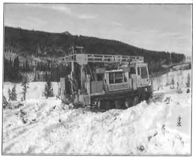
Left: A larger track mounted drilling rig.
